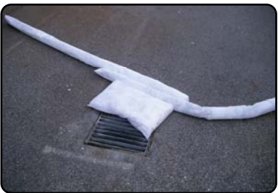
Spill Kit components being used to protect a stormwater drain
