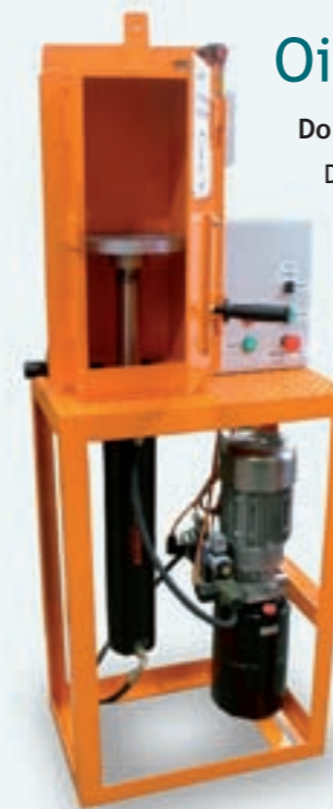
▲ Oil Filter Crusher shown without the protective covering around the hydraulic motor and tank
